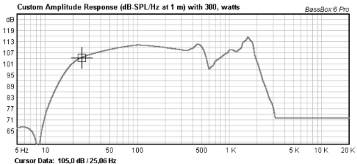
The response of the system will be extended to 20 Hz but the efficiency is lower than the previous. Inspecting the cone displacement results in the following result.
