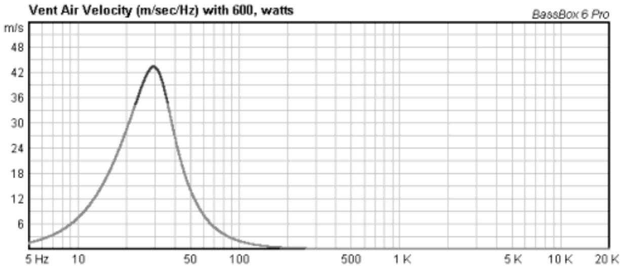
This means that a larger diameter of port is needed, which will require that the port is longer. Using a 90 mm port and 510 mm of length turns out to be a good choice:
