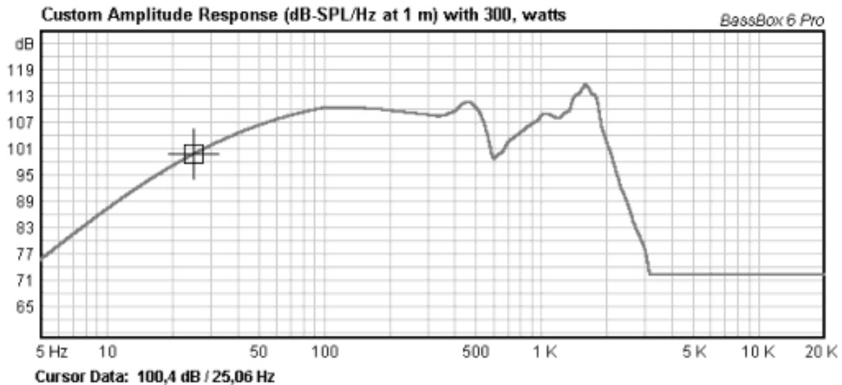
From the graph we see that it is necessary to boost by about 10 dB at 25 Hz with a low pass slope of 12 dB/oct. to achieve a flat response.
