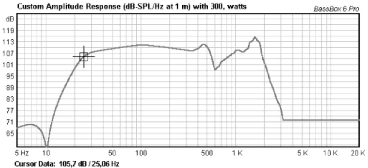
At 25 Hz the maximum is around 106 dB, but we need to inspect the cone and slave excursion before proceeding with the design.
