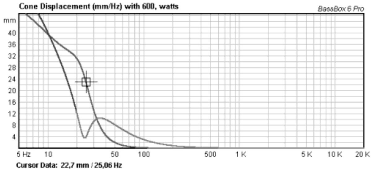
From this simulation we see that the maximum excursion of the driver is well within the linear limits down to about 20 Hz where the linearity limit of 12.5 mm is reached.
